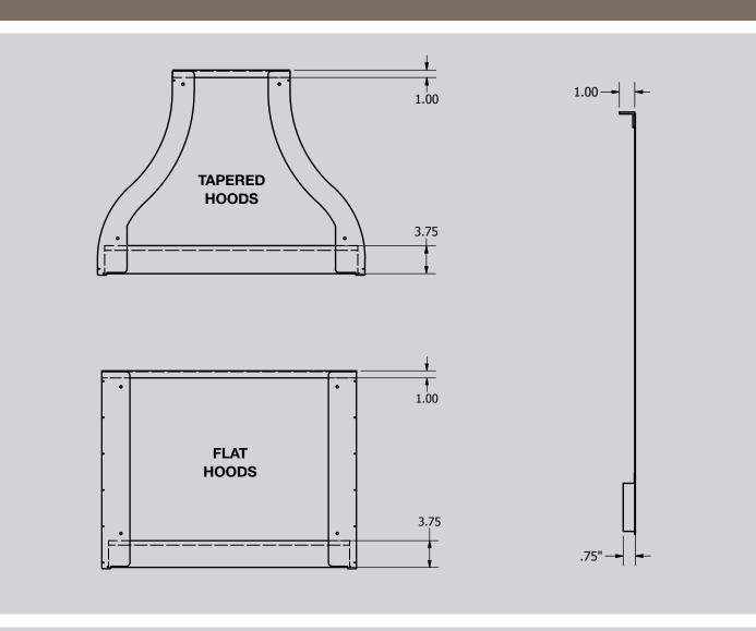
Haube hoods were designed to provide a flexible amount of space for a variety of ducting situations. Each one allows the options to duct through the top or back of the hood. This allows for more ducting options for an easier installation process. The sooner your hood is up, the sooner you can enjoy your thoughtfully crafted kitchen.
